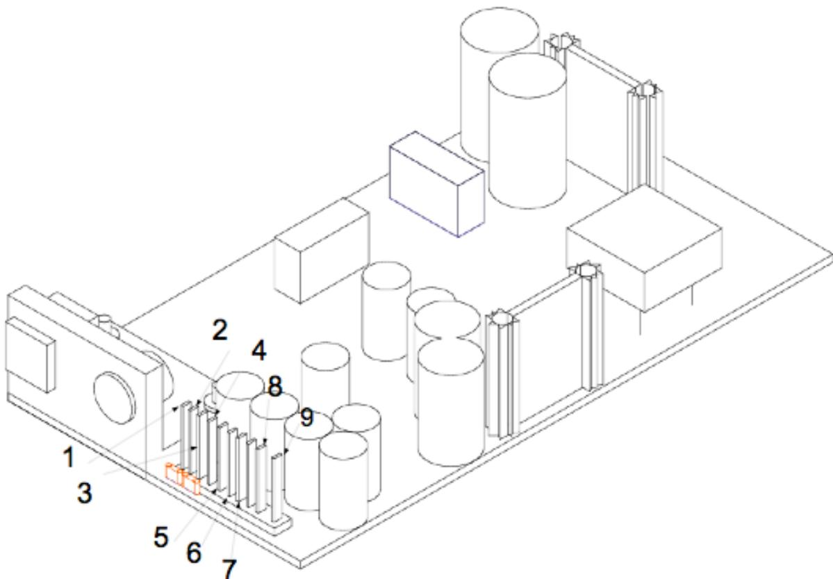
The diagram above illustrates the pin numbers that will be referenced on the next page. The following is data that is typical of a good power supply. Remember that each low voltage supply is different and a difference of a volt or so will not influence the total performance of the supply. The following chart gives approximate values for the voltage differences between the Leads. If a spot is listed as NA, then its value is not important for the supply.
