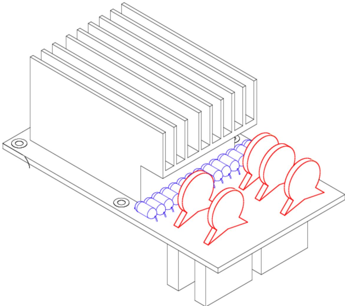
The high voltage pod requires other voltage to power it; it then amplifies that voltage and exports it through the cable connectors at its base. There are two options for providing a voltage to the HV pod. First, it is possible that CROP has a low voltage power supply strictly for this use (we did in my days). This is the easiest method.
