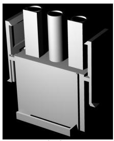
This is an illustration of the voltage head used in CROP. Notice the strip of plastic down the length of the rectangular portion. This line indicates the space in which the **High Voltage** wire is placed.
